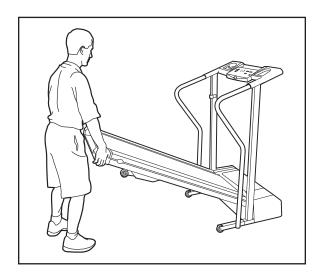
Move your right hand to the position shown and hold the treadmill firmly. Raise the treadmill until the storage latch closes over the catch. Make sure that the storage latch is fully engaged over the catch.
